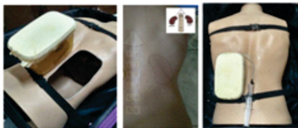
Figure 4. Kidney phantoms on torso mannequin.
